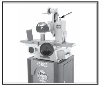
Figure 5. Lifting location.
